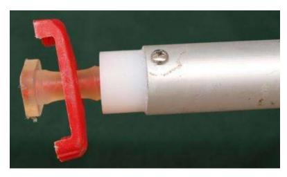
Boats produced **after 2012**: simply wind the adjuster eye in or out as needed. Remember to tighten the lock nut up after adjustment.
