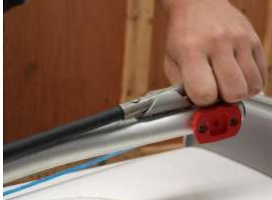
3. Align the lockdown pin with the hole and squeeze the end of the lock down rod and the tiller arm to press it into position.
