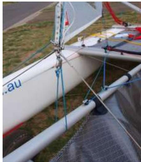
5. Connect the 2 shock cords at the end of the chute to the loops under the trampoline. This should keep the chute taught. These pass UNDER the Cunningham lines.
