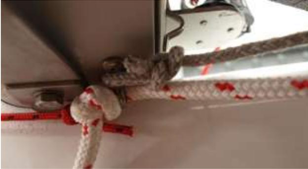
4. Before racing you should be sure that the reinforced area of the tack line is in the cleat when the tack is fully pulled out, adjust this by shortening or lengthening the knot at the tack of the spinnaker.
