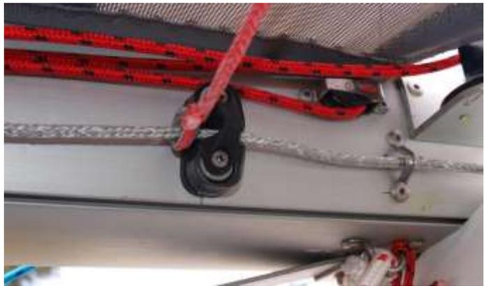
2. Pass the line between the tramp and hull to the turning pulley on the outside of the beam and then pass it through the eyelet in the tramp.
