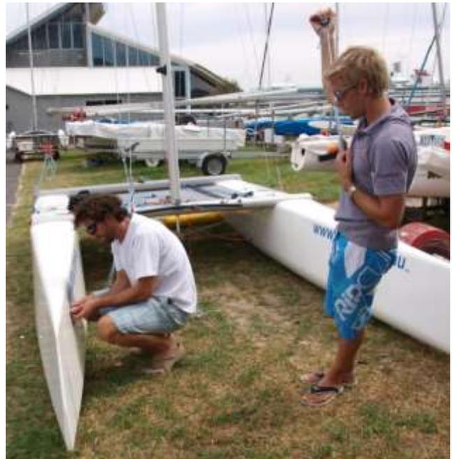
10. Set the fore stay to the appropriate hole on the bridle tube for the required mast rake, as per the tuning guide.
