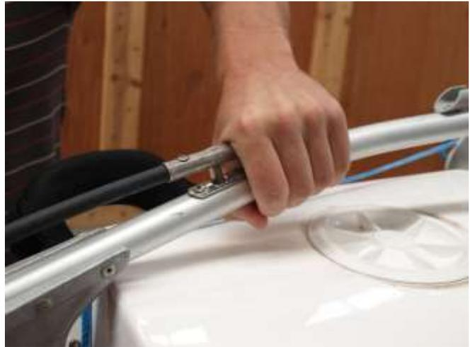
4. The lockdown rod should be set to the correct length from the factory. If for any reason you have to adjust it, simply undo the lock nut and rotate the rod to shorten or lengthen it. The rod should be under a medium amount of compression when in the lockdown position, such that there is a small bow in the rod.
