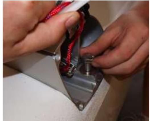
3. Wipe all dirt and grease from the beam pad before sitting the beam on. Make sure the beams are facing the correct way. The rear beam should have the traveler saddles facing backwards. Apply grease to the threaded part of all bolts before inserting them into the hull. Get all the bolts started before tightening any of the bolts. We recommend beginning with the inner front beam bolt. If a particular bolt is being difficult to fit. Release all the beam bolts and fit this bolt first.
