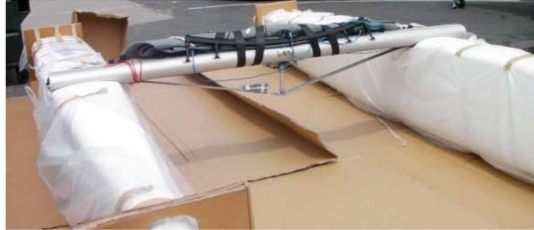
2. The beams will come from the factory pre-rigged and ready to go onto the boat. The shorter bolts and smaller washers are for the outer locations and the longer bolts and bigger washers for the inner locations. To access the outer bolt holes you will have to remove the plastic end caps from the beams with a Phillips head screwdriver, don't undo any of the shock cords on the front beam as they are already in the correct position.
