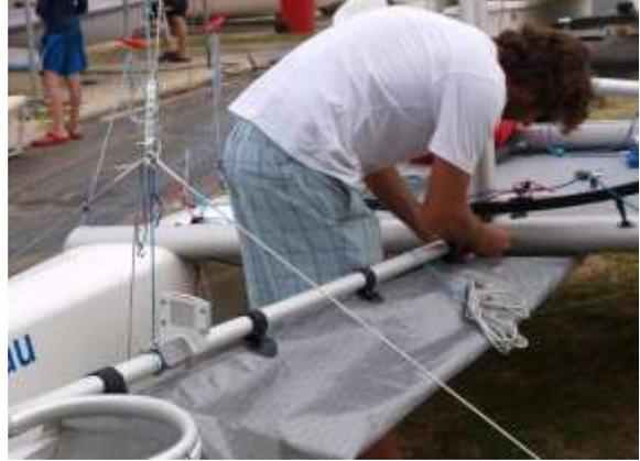
2. Assure that the knots on both bow braces are the same length. Connect the front braces to the bow by passing a loop through the hole in the bow and then pass the knotted tail through the loop on the outside to prevent the loop coming back through. Work this firm so it will not move during sailing.
