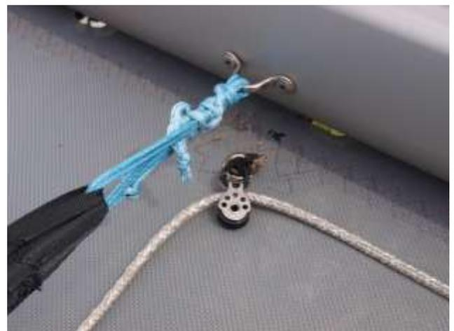
2. Pass the retrieval line through the eyelet in the bottom of the chute and use the tiller extension to pull it up and out by poking the extension down and tying the line to it.
