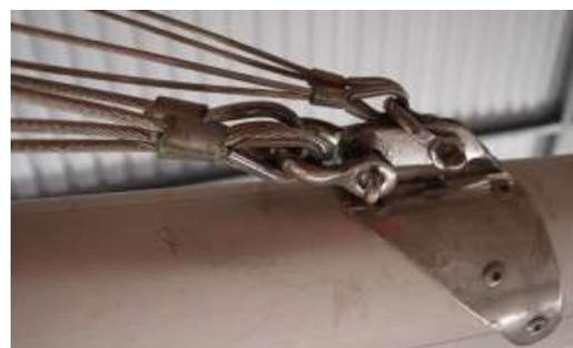
4. Connect the side stays to the corresponding chain plates, with the Stamaster adjusters at maximum length.
