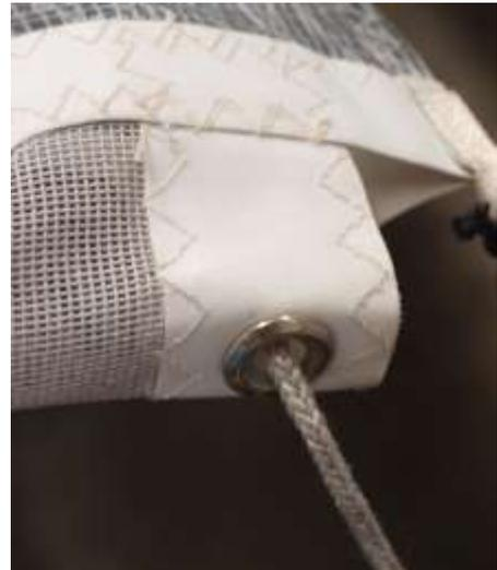
3. Tie the retrieval line to the bridle until you are ready to attach the spinnaker.
