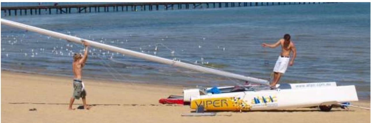
8. When the mast is vertical allow the mast to rotate so that sail groove now faces backwards. **DO NOT** let the mast rotate until it is vertical.
