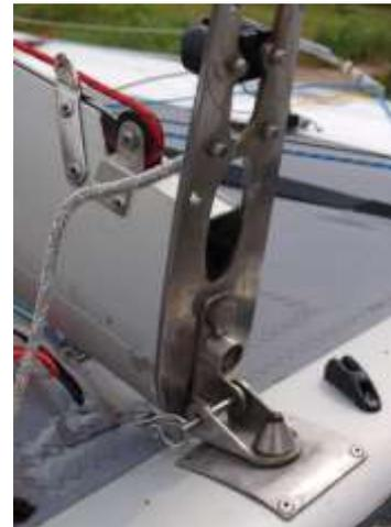
7. Walk the mast up from the stern, you will need to step onto the trap or pass the mast to a 3<sup>rd</sup> person already on the deck to complete this. At the same time the 2nd person should be pulling the mast up using one of the trapeze wires.
