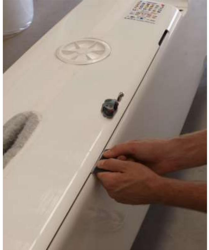
6. To fit the trampoline to the main beam, remove the end plate from the front beam and slide the trampoline into the front beam groove refitting the end plate once the tramp is in place.
