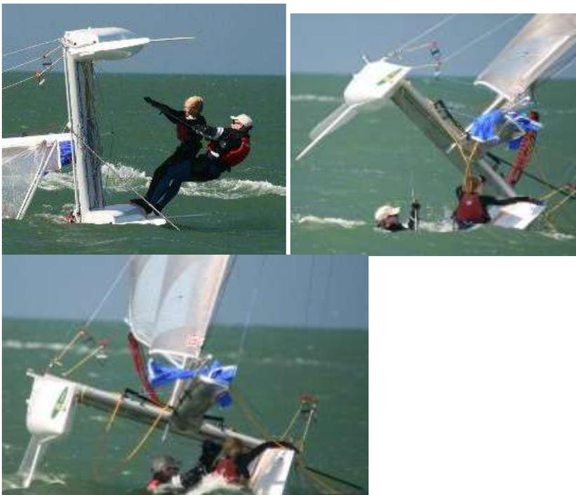
As soon as the boat is upright, grab the dolphin striker. This will, not only keep the boat from capsizing to the other side, but will also keep you and the crew connected to the boat. Climb aboard over the front beam and use the dolphin striker as a step.
