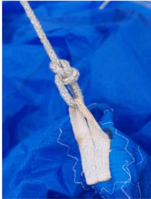
4. The spinnaker sheets are attached by hitching the connecting loop in the middle of the spinnaker sheet through the eyelet in the clew of the spinnaker.
