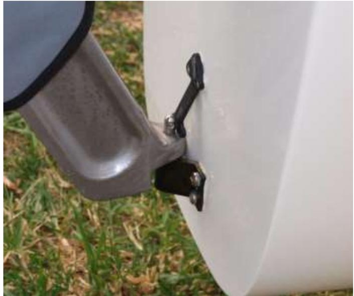
Connect the crossbar on the pins with the retaining clip.
