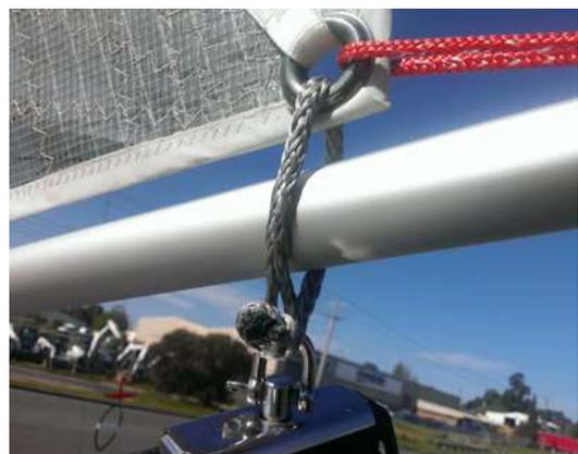
Connect the Cunningham to the sail. This consists of 2 single tack pulleys that go either side of the main sail and a single pulley that is attached to a bracket just above the base of the mast. Run the rope loop from one of the clew pulleys through the clew eyelet of the main sail and through the other clew pulley and run the knotted end of the rope through the rope loop.
