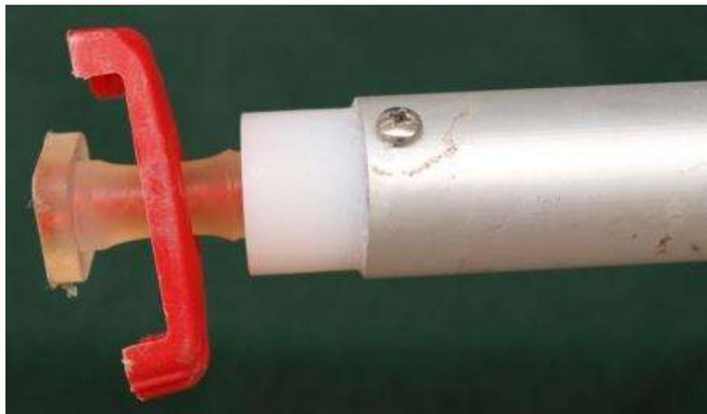
Boats produced **after 2012**: simply wind the adjuster eye in or out as needed. Remember to tighten the lock nut up after adjustment.
