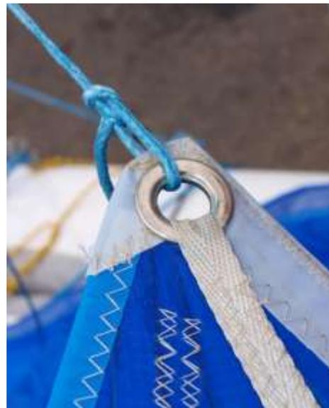
3. Untie the retrieval from the bridal and pass it through the retrieval points on the spinnaker and tie it off at the top retrieval point.
