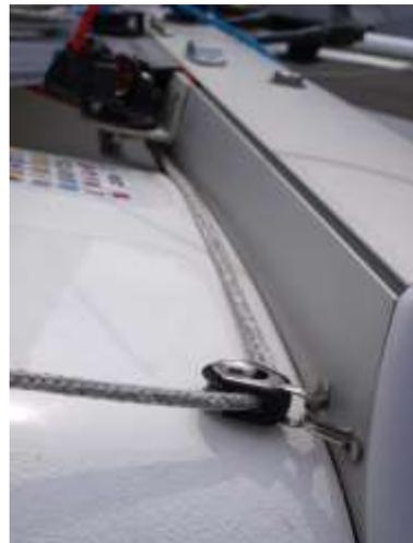
3. On the underside of the tramp, pass the tack line through the ring on the spinnaker retrieval shock cord and finish by tying it off at starboard righting rope saddle on the main beam. These lines should pass on top of all other shock cords.
