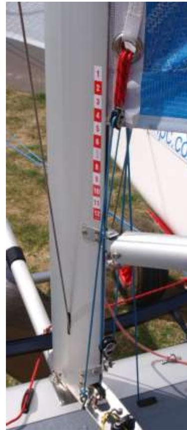
The clip on the end of the downhaul rope hooks into the hole the mast spanner.
